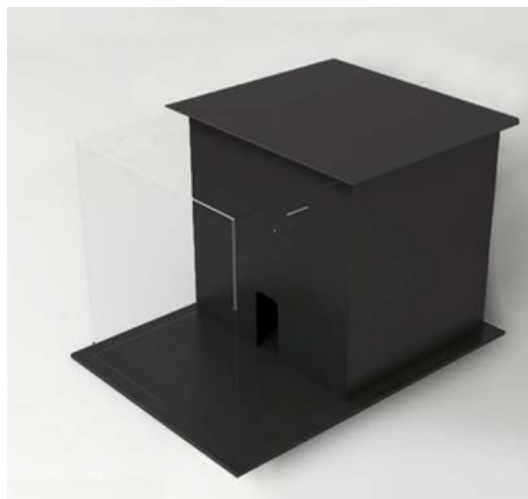
An example of a light-dark box for mice. Credits: He, S. and Corscadden, L. (2022). Maze Engineers.
