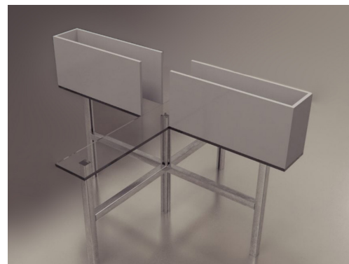
A standard elevated plus maze. Credits: He, S. and Corscadden, L. (2022). Maze Engineers.
