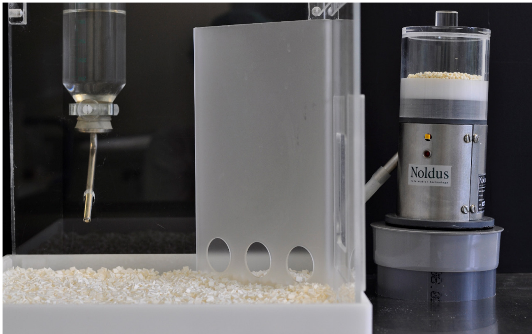
PhenoTyper home cage monitoring system can come equipped with a number of hardware solutions. Including a Cognition Wall (by Sylics) and a food pellet dispenser. Photo credits: Sylics.
